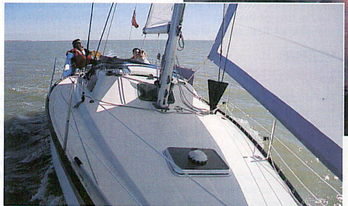
A short coachroof leaves an almost flush foredeck. The keel's lifting line emerges through a pulley just abaft the mast and is led back to a winch.
